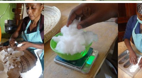
From left: fluff is pressed into a pad; interior pad is covered in biodegradable plastic and cut; after bio degradable adhesives are affixed to the pad, it will be sanitized.
